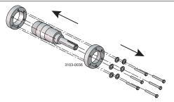
Study the instructions carefully. The items refer to the parts list and service kits section. Lubricate the rubber seals before fitting them.
