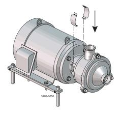
Study the instructions carefully. The items refer to the parts list and service kits section. Lubricate the rubber seals before fitting them.
