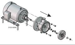
Study the instructions carefully. The items refer to the parts list and service kits section. Lubricate the rubber seals before fitting them.
