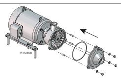
Study the instructions carefully. The items refer to the parts list and service kits section. Lubricate the rubber seals before fitting them.
