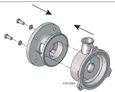
Study the instructions carefully. The items refer to the parts list and service kits section. Lubricate the rubber seals before fitting them.
