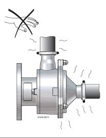
Never run the pump with both the suction side and the pressure side blocked.
